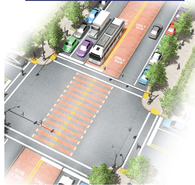
MEDIAN BUS LANE
